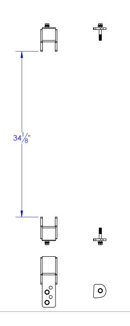
RISER KIT OPTION IS NOT SUPPLIED IN THIS KIT BUT MUST BE USED FOR ALL ELECTRIC BUCHER SOLENOID VALVES
